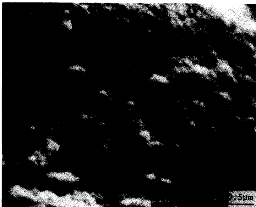
FIG. 4. Scanning electron micrograph of NiO/ \alpha -Al 2 O 3 -1050 at \times 20,000 .
